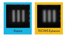
USAF target images (0.00  $\mu m)$  SA model cornea using 3mm aperture
